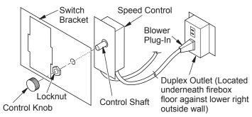
Figure 26 - Attaching Speed Control to Firebox
